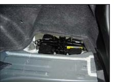
The Jack and it's mounting foam will be removed from the compartment on the passengers side of the trunk floor.
